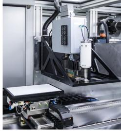
2D inkjet printing test bench including vacuum table and curing mechanism (UV, IR).
